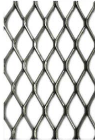
REAL STEEL Expanded Metal Flat 3/4" X #9ga (opening size: Lwo 1.63" Swo .56")
