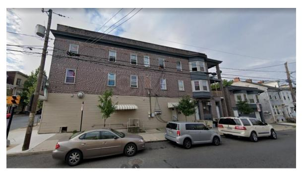
**Proposed alterations:** It is proposed to renovate east façade into convenience store. The existing exterior finish on the 1<sup>st</sup> floor, east façade, will be removed. A new aluminum storefront with opaque glass panels will be installed. The existing brick façade will be repaired and repointed as necessary.
