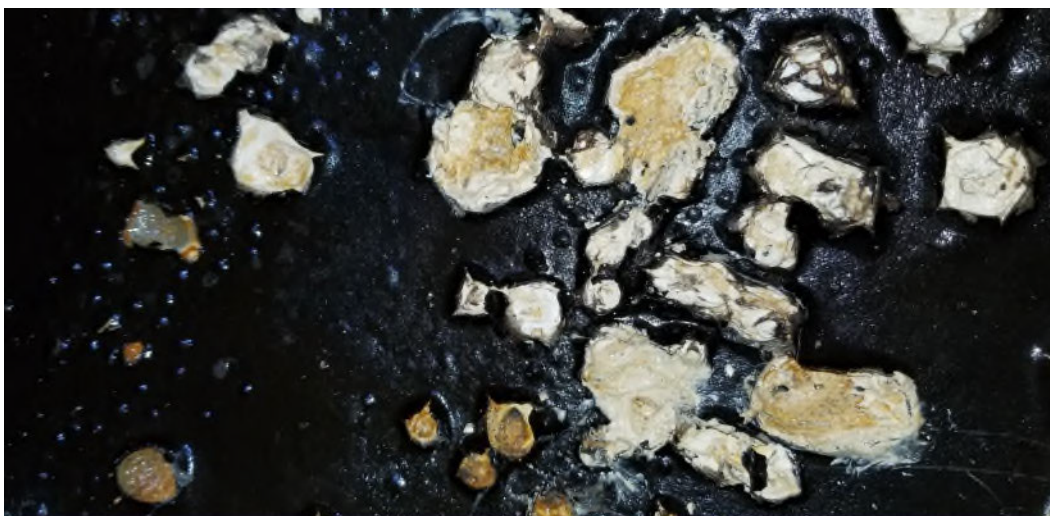
Figure 24 - ARV 6 toward ARV 7 - Blisters in Coating
