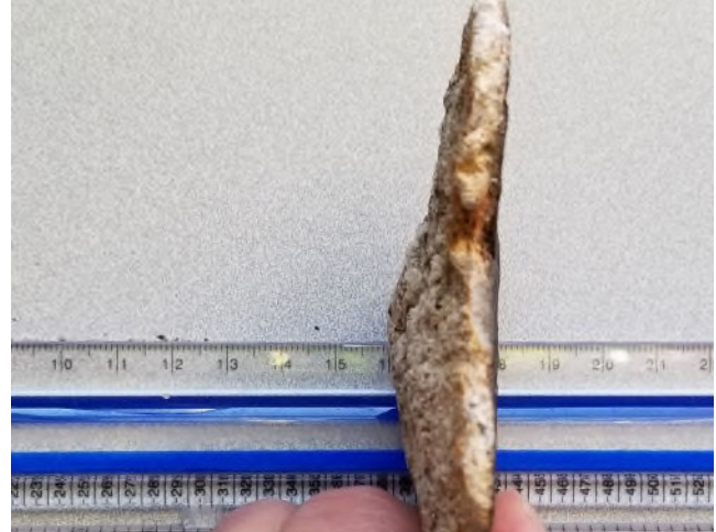
Figure 27 - Shard of PCCP Inner Liner Mortar and Coal Tar Coating near ARV 8
