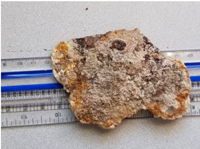
Figure 27 - Shard of PCCP Inner Liner Mortar and Coal Tar Coating near ARV 8
