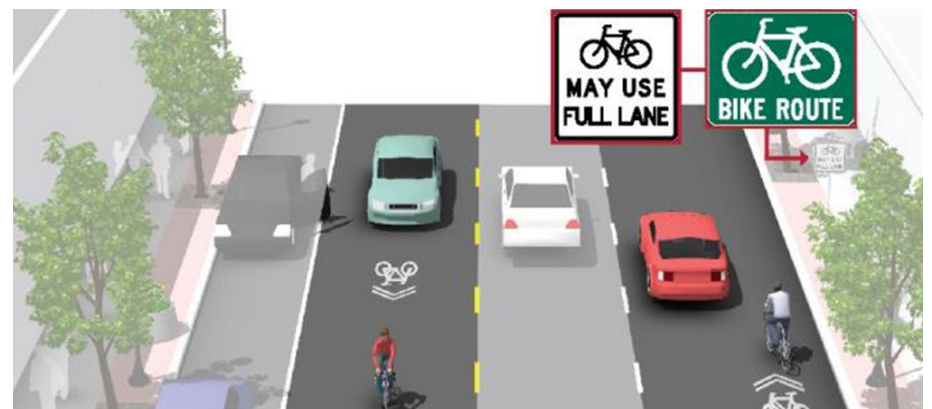
Top: Examples of sharrows. Bottom: Example of a Shared Roadway using shared lane markings and signage. Source: NACTO.
