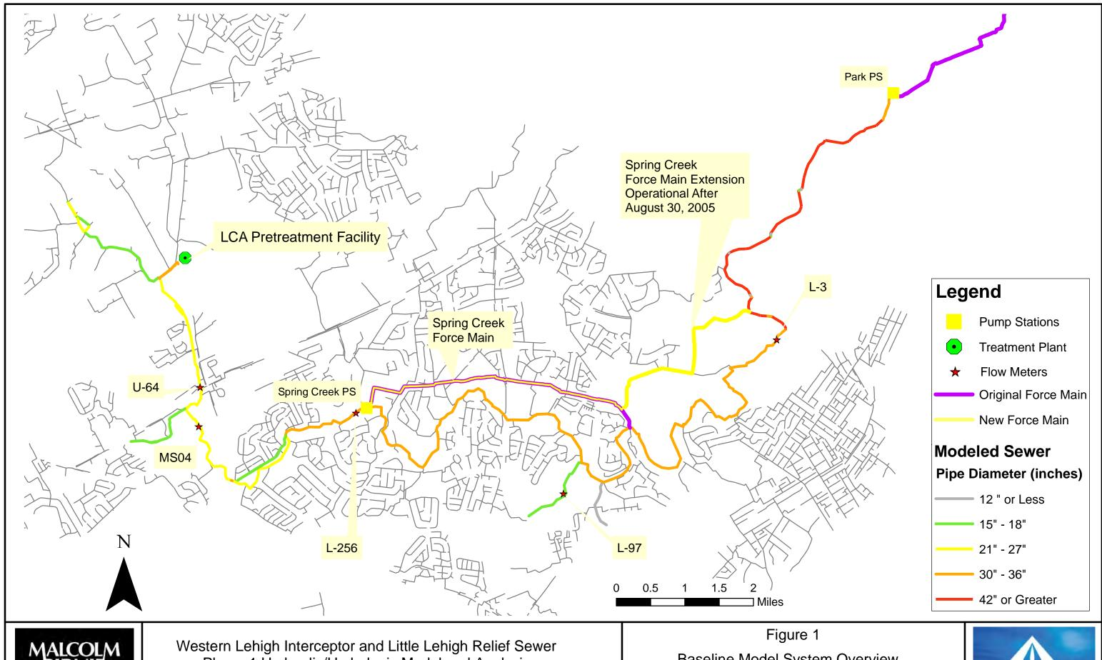
Phase 1 Hydraulic/Hydrologic Model and Analysis
