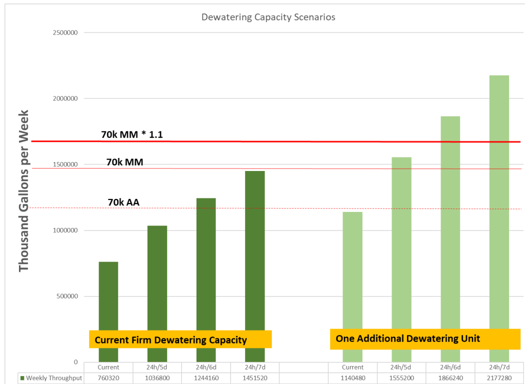
Figure 5 – Dewatering Capacity Analysis
