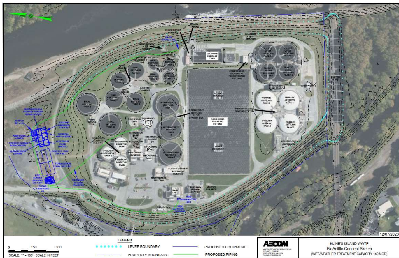
Figure 3: Site Arrangement Drawing for High-rate Treatment Approach at 140 MGD.
