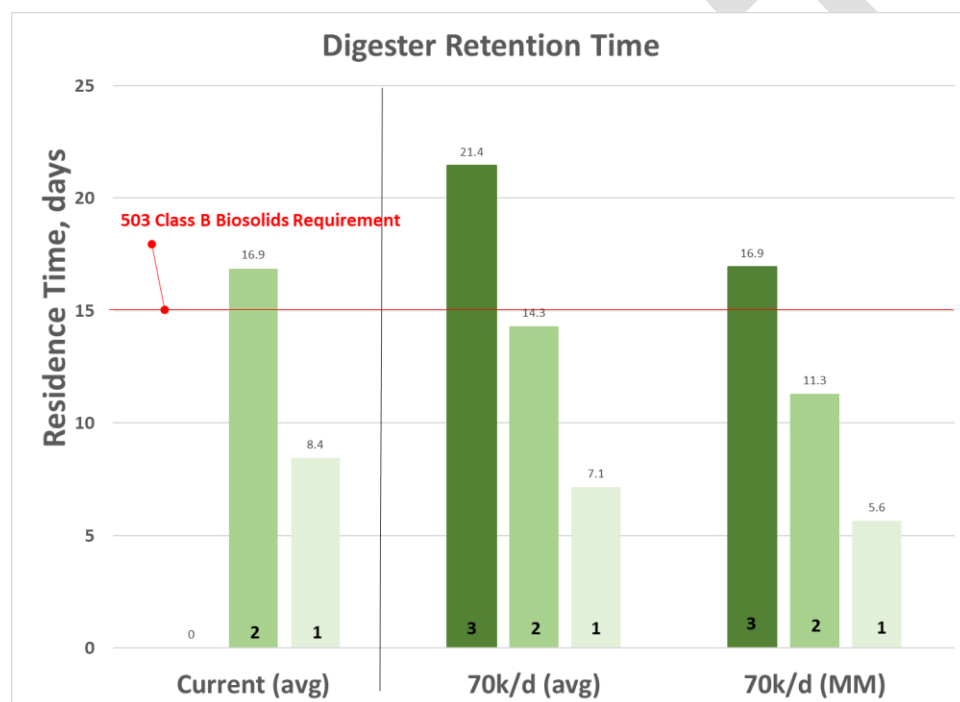
Figure 4 – Digester Capacity Analysis based on Retention Time
