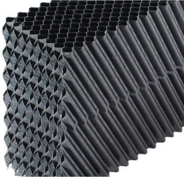
Figure 7. Brentwood Industries CF-900 cross flow media (specific surface area = 48 ft 2 /ft 3 )
