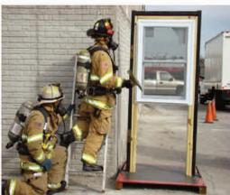
Figure 13: Second Story Window Breakage Prop
