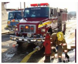
Figure 16: Connecting to the Hydrant
